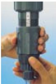
The injection rate is set by lining up the top of the adjusting sleeve with the desired ratio on the scale. The amount of injected concentrate is proportional to the amount of water coming into the Dosatron :
